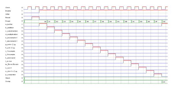
Fig. 6 TCU Timing Diagram of Processor ALU in SDR/SOR
