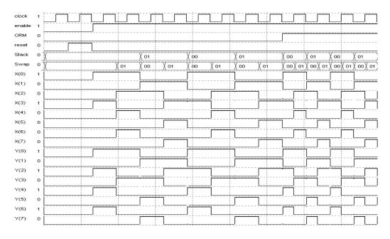
Fig. 5 Timing Diagram of Stack-Swap circuit of Memory-Processor ALU in Dual-Mode
