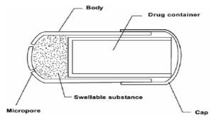
Fig 1: Time-controlled capsule for colonic delivery <sup>59</sup>
