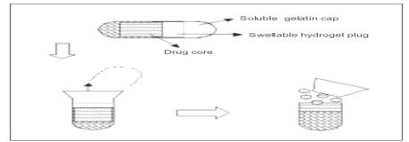
Fig. 2: Design of Pulsincap® system.
