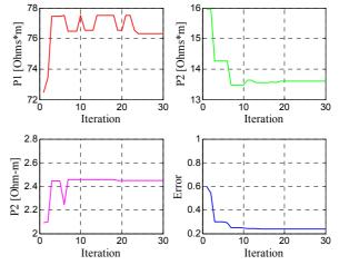
Fig. 3. Convergence of two-layer earth parameters.
