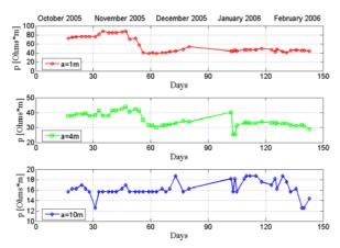
Fig. 4. Variation of the apparent soil resistivity upon the distance of the auxiliary electrodes (a=1m, a=4m and a=10m).
