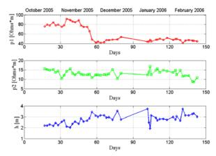
Fig. 5. Variation of two-layer earth parameters during the year.
