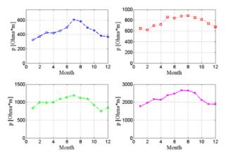
Fig. 2. Variation of the apparent soil resistivity during the year at various areas (a=10m).
