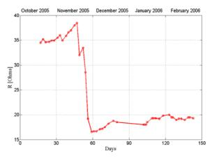
Fig. 6. Variation of grounding system resistance during the year.
